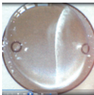
Fig 2. Copper carbonate precipitates in a 2cm puddle of water
