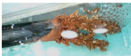
Fig 1. Copper growing from the cathode during electrolysis
