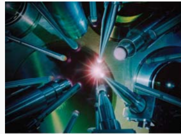
The international inertial confinement fusion community, including LLNL researchers, uses the OMEGA laser at the University of Rochester's Laboratory for Laser Energetics to conduct experiments and test target designs and diagnostics. The 60-beam OMEGA laser at the University of Rochester has been operational since 1995.
